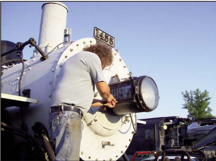
Ira Pollack replaces the glass and the stenciled numerals on the #1455's number board.
