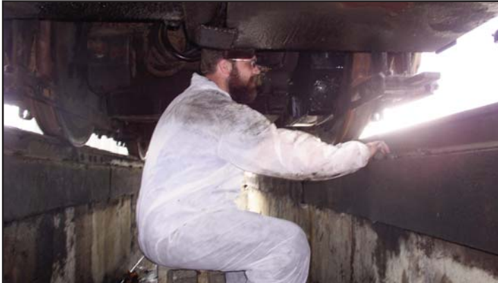
CMO Justin Chapin reinstalled the traction motor gear case, all patched and shiny, on the SW-8 Pfizer locomotive.
