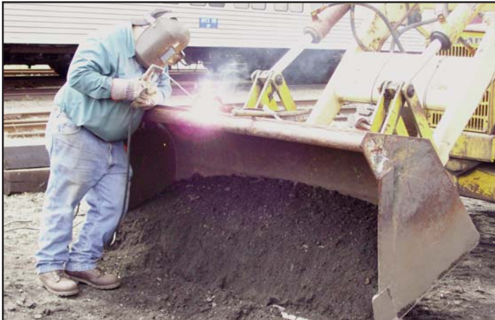
Earlier this year Bob Pitcher welded a damaged hook on to the backhoe.
