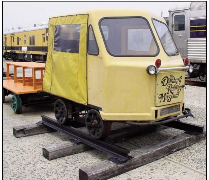
The Woodings track car makes its home on the center platform of the DRM railyard.
