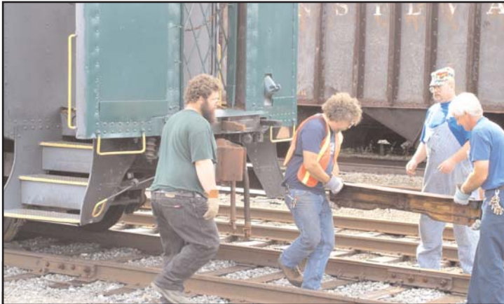
Above: (left to right) Justin Chapin, Ira Pollack, Glenn Miller, and Bruce Van Wyk carry a buffer to be replaced at the end of a coach. Left: Don Konen (top), Justin Chapin, and Bruce Van Wyk carefully lift the buffer into place. An additional coach was needed
